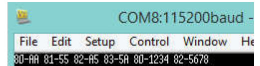
4 times a Byte to 80, 81, 82 and 83, and 2 times a Word to port 80 and 82 BIOS POST code example
