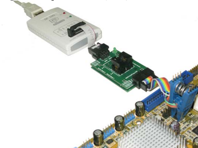
Fig 3: Backup Boot Flash (BBF) connected to SF100
