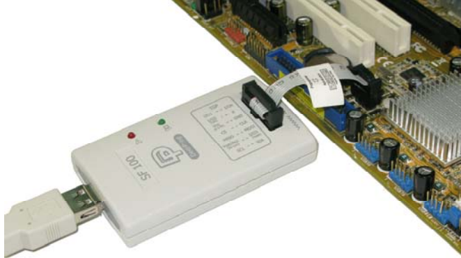
Fig 2: SF100 connected to the application pin header
