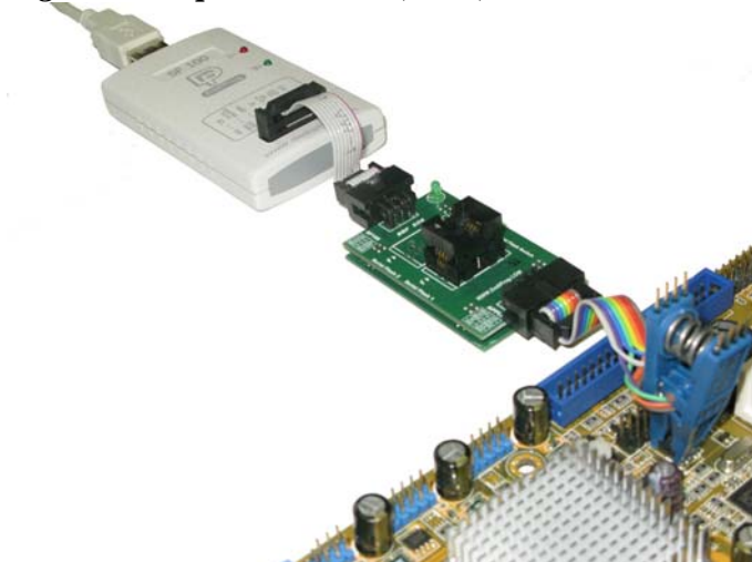
Fig 3: Backup Boot Flash (BBF) connected to SF100
